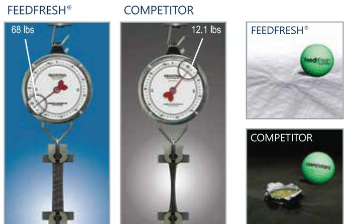
Scale Comparison: The amount of force required to pull cover materials near the breaking point.
