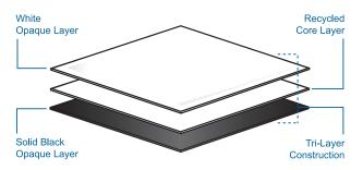
Virgin Grade Outer Layer Resins = Stable Outdoor Exposure Recycled Core Resins = Economical Green Alternative Tri-layer Construction = Excellent Tear & Puncture Strengths
