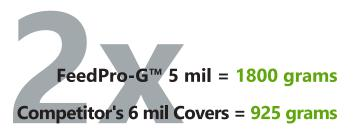
Elmendorf Tear Test MD - ASTM 1922 Competitor Covers based on average of four specimens
