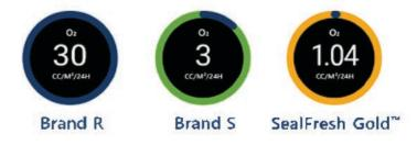
SealFresh® Gold™ Compared against two leading barrier silage cover films according to ASTM D-3985/DIN 53380-3 at 21% Oxygen Permeability
