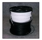
VIAFLEX Welding Rod is used for field seaming, repairs and detail work, such as installing pipe boots. Packaged in 25 lb spools, it is available in 4mm and 5mm sizes to fit most brands of extrusion guns. VIAFLEX Welding Rod is made from a thermally UV stabilized LLDPE resin and is available in both black and white to correspond with the color of geomembranes being utilized.
