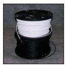
VIAFLEX Welding Rod is used for field seaming, repairs and detail work, such as installing pipe boots. Packaged in 25 lb spools, it is available in 4mm and 5mm sizes to fit most brands of extrusion guns. VIAFLEX Welding Rod is made from a thermally UV stabilized LLDPE resin and is available in both black and white to correspond with the color of geomembranes being utilized.
