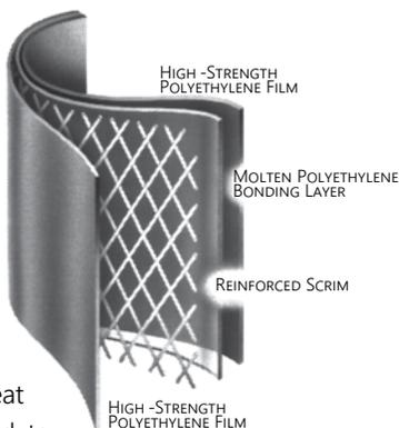
A layer of polyester scrim reinforcement placed between these plies greatly enhances tear resistance and increases service life. DURA♦SKRIM® R20WWK is reinforced with a high strength scrim reinforcement laid in a diagonal pattern spaced 3/8" apart for uniform tear resistance in both machine and transverse directions with an additional machine direction scrim every 3" across the width for increased stability.
